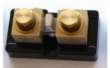
Shunts are usually rated by current and voltage drop. For example, a Riedon RSB-300-50 is rated for 300A and 50mV. If you see a shunt rated by current and resistance, you can calculate its voltage drop as V=IR (voltage = current × resistance).
